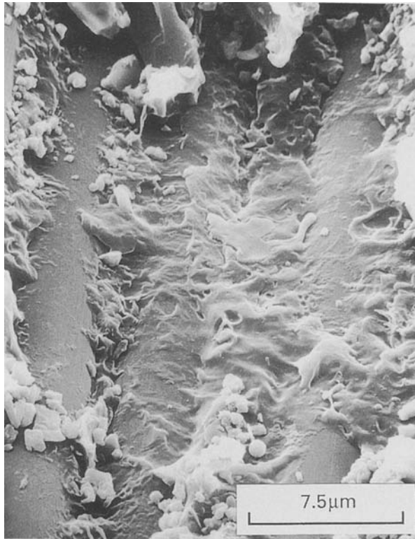
Figure 4 Composite surface after delamination of the HA-coating. The surface of certain carbon fibres have partially matrix-free domains.
